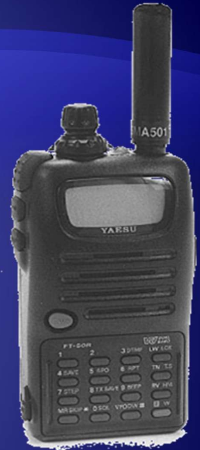
Comet SMA- 501 0 dBi at \frac{1}{4} wave - Not!
